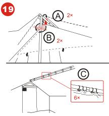
Hang the inner tent to the ridge pipe, start first with only one hook at each end of the ridge pipe (A),then attach the inner tent to the upright poles with the laces(B), and then place the remaining 6 hooks on the ridge pipe(C).
