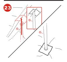
Place the central pole; make sure the base plate is located where the ground sheet is reinforced.
