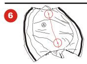
place the outer tent canvas inside up to make the ridge line visible. To identify the ridge line, look for the two Velcro sleeves, and also see the two triangular vents at each end of the ridge.
