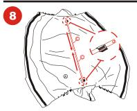
Assemble the ridge pipe and place it on the tent canvas, attach it with the two Velcro sleeves.
