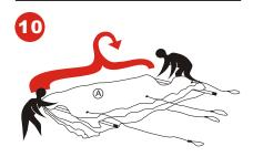
Fold back the outer tent canvas on the previously installed pipes.
