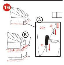
(A): Once the shape of the outer tent is appropriate, fix the bottom of the walls to the ground with 22 pegs, from outside.
