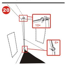
Hang the inner tent side walls to the side poles, using the 16 hooks and the 10 D-rings at the top and the 6 at bottom of the walls. Start from the middle, and finish by the door side.
