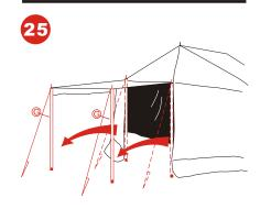
Outer tent doors can be used as awnings by moving the door poles, the door guy ropes and the pegs.
