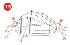
Place the remaining 6 pegs, attach and tension moderately all the guy ropes.
