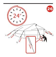
Check regularly the tensioning of the guy ropes and adjust if needed.
